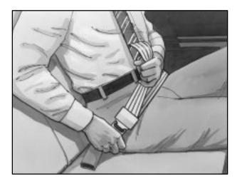
To make the belt shorter, pull its free end as shown until the belt is snug.
